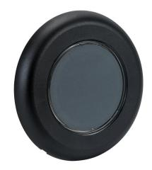
Captron Caneo Series41 Standard capacitive pushbutton sensor switch, IP69K, 27-60mm, dynamic, polycarbonate bezel, semi-automatic LED control, Operator: black, 99.8mm. Requires 4-pin female M12 cable.
