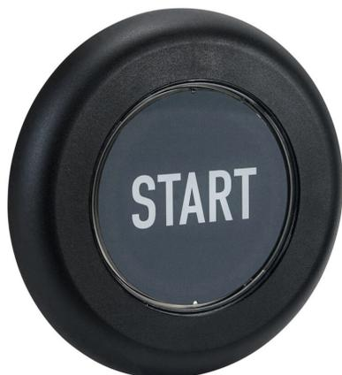
Captron Caneo Series41 Standard capacitive pushbutton sensor switch, IP69K, 27-60mm, dynamic, polycarbonate bezel, manual LED control, Operator: black, 99.8mm, operator text "START", white. Requires 5-pin female M12 cable.
