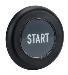
Captron Caneo Series41 Standard capacitive pushbutton sensor switch, IP69K, 27-60mm, dynamic, polycarbonate bezel, semi-automatic LED control, Operator: black, 99.8mm, operator text "START", white. Requires 4-pin female M12 cable.
