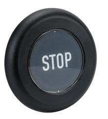
Captron Caneo Series41 Standard capacitive pushbutton sensor switch, IP69K, 27-60mm, dynamic, polycarbonate bezel, semiautomatic LED control, Operator: black, 99.8mm, operator text "STOP", white. Requires 4-pin female M12 cable.
