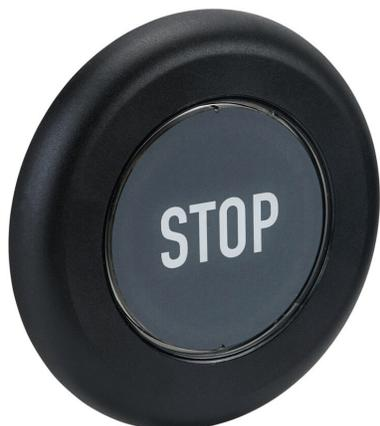
Captron Caneo Series41 Standard capacitive pushbutton sensor switch, IP69K, 27-60mm, dynamic, polycarbonate bezel, automatic LED control, Operator: black, 99.8mm, operator text "STOP", white. Requires 3-pin female M12 cable.
