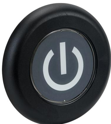
Captron Caneo Series41 Standard capacitive pushbutton sensor switch, IP69K, 27-60mm, dynamic, polycarbonate bezel, manual LED control, Operator: black, 99.8mm, operator text "power symbol", white. Requires 5-pin female M12 cable.
