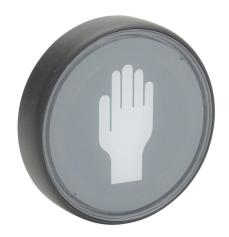
Captron Caneo Series40 Puck capacitive pushbutton sensor switch, IP69K, 22mm, dynamic, polycarbonate bezel, automatic LED control, Operator: black, 68mm, operator text "hand symbol", white. Requires 4-pin female M12 cable.
