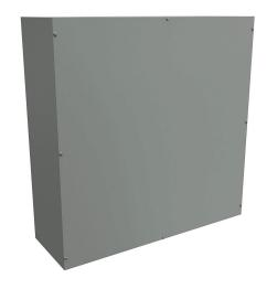
Hammond enclosure, NEMA 1, 36 x 36 x 12in (HxWxD), wall mount, carbon steel, ANSI 61 gray, powder coat finish, screw cover.
