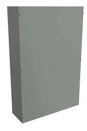
Hammond enclosure, NEMA 1, 36 x 24 x 8in (HxWxD), wall mount, carbon steel, ANSI 61 gray, powder coat finish, screw cover.
