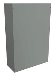
Hammond enclosure, NEMA 1, 36 x 24 x 10in (HxWxD), wall mount, carbon steel, ANSI 61 gray, powder coat finish, screw cover.
