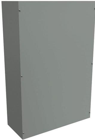
Hammond enclosure, NEMA 1, 36 x 24 x 10in (HxWxD), wall mount, carbon steel, ANSI 61 gray, powder coat finish, screw cover.
