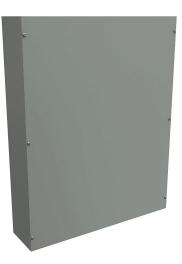
Hammond enclosure, NEMA 1, 30 x 24 x 6in (HxWxD), wall mount, carbon steel, ANSI 61 gray, powder coat finish, screw cover.
