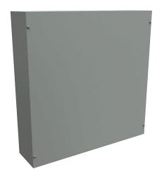
Hammond enclosure, NEMA 1, 24 x 24 x 6in (HxWxD), wall mount, carbon steel, ANSI 61 gray, powder coat finish, screw cover.
