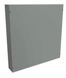
Hammond enclosure, NEMA 1, 24 x 24 x 4in (HxWxD), wall mount, carbon steel, ANSI 61 gray, powder coat finish, screw cover.
