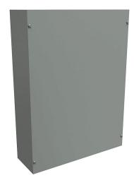
Hammond enclosure, NEMA 1, 24 x 18 x 6in (HxWxD), wall mount, carbon steel, ANSI 61 gray, powder coat finish, screw cover.
