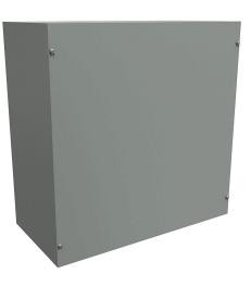
Hammond enclosure, NEMA 1, 20 x 20 x 10in (HxWxD), wall mount, carbon steel, ANSI 61 gray, powder coat finish, screw cover.
