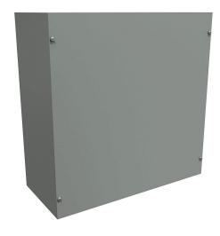
Hammond enclosure, NEMA 1, 18 x 18 x 8in (HxWxD), wall mount, carbon steel, ANSI 61 gray, powder coat finish, screw cover.
