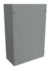
Hammond enclosure, NEMA 1, 18 x 12 x 6in (HxWxD), wall mount, carbon steel, ANSI 61 gray, powder coat finish, screw cover.
