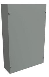
Hammond enclosure, NEMA 1, 18 x 12 x 4in (HxWxD), wall mount, carbon steel, ANSI 61 gray, powder coat finish, screw cover.
