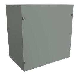
Hammond enclosure, NEMA 1, 12 x 12 x 8in (HxWxD), wall mount, carbon steel, ANSI 61 gray, powder coat finish, screw cover.
