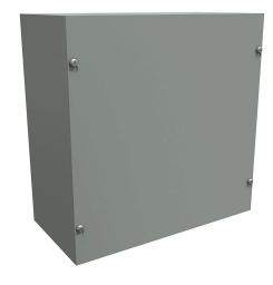
Hammond enclosure, NEMA 1, 12 x 12 x 6in (HxWxD), wall mount, carbon steel, ANSI 61 gray, powder coat finish, screw cover.
