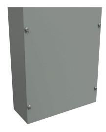
Hammond enclosure, NEMA 1,  $12 \times 10 \times 4$ in (HxWxD), wall mount, carbon steel, ANSI 61 gray, powder coat finish, screw cover.
