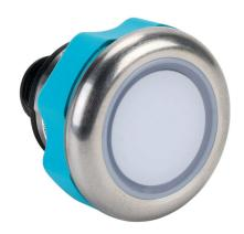
Captron Caneo Series10 Stainless Steel capacitive pushbutton sensor switch, IP69K, 22mm, static, stainless steel bezel, semi-automatic LED control, Operator: white, 30mm. Requires 4-pin female M12 cable.
