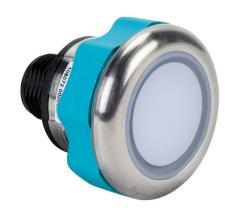
Captron Caneo Series10 Stainless Steel capacitive pushbutton sensor switch, IP69K, 22mm, dynamic, stainless steel bezel, semi-automatic LED control, Operator: white, 30mm. Requires 4-pin female M12 cable.
