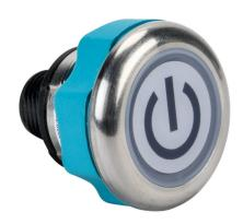
Captron Caneo Series10 Stainless Steel capacitive pushbutton sensor switch, IP69K, 22mm, static, stainless steel bezel, semi-automatic LED control, Operator: white, 30mm, operator text "power symbol", black. Requires 4-pin female M12 cable.
