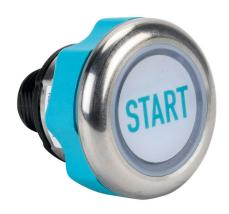
Captron Caneo Series10 Stainless Steel capacitive pushbutton sensor switch, IP69K, 22mm, static, stainless steel bezel, semi-automatic LED control, Operator: white, 30mm, operator text "START", green. Requires 4-pin female M12 cable.
