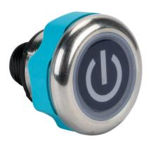
Captron Caneo Series10 Stainless Steel capacitive pushbutton sensor switch, IP69K, 22mm, static, stainless steel bezel, semiautomatic LED control, Operator: black, 30mm, operator text "power symbol", red/green illuminated. Requires 4-pin female M12 cable.
