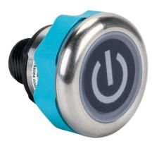
Captron Caneo Series10 Stainless Steel capacitive pushbutton sensor switch, IP69K, 22mm, static, stainless steel bezel, semiautomatic LED control, Operator: black, 30mm, operator text "power symbol", green/red illuminated. Requires 4-pin female M12 cable.
