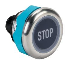
Captron Caneo Series10 Stainless Steel capacitive pushbutton sensor switch, IP69K, 22mm, dynamic, stainless steel bezel, semi-automatic LED control, Operator: black, 30mm, operator text "STOP", red/green illuminated. Requires 4-pin female M12 cable.
