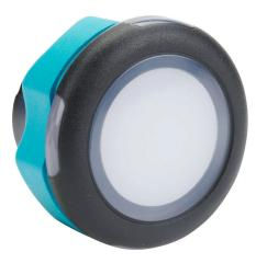
Captron Caneo Series10 Standard capacitive pushbutton sensor switch, IP69K, 22mm, dynamic, polycarbonate bezel, semiautomatic LED control, Operator: white, 30mm.
