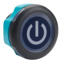
Captron Caneo Series10 Standard capacitive pushbutton sensor switch, IP69K, 22mm, static, polycarbonate bezel, semi-automatic LED control, Operator: black, 30mm, operator text "power symbol", green/red illuminated.
