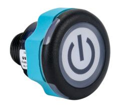
Captron Caneo Series10 Standard capacitive pushbutton sensor switch, IP69K, 22mm, static, polycarbonate bezel, semi-automatic LED control, Operator: white, 30mm, operator text "power symbol", black. Requires 4-pin female M12 cable.
