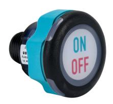
Captron Caneo Series10 Standard capacitive pushbutton sensor switch, IP69K, 22mm, toggle, polycarbonate bezel, semi-automatic LED control, Operator: white, 30mm, operator text "ON/OFF", green/red. Requires 4-pin female M12 cable.
