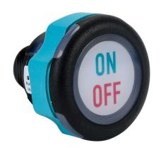
Captron Caneo Series10 Standard capacitive pushbutton sensor switch, IP69K, 22mm, dynamic, polycarbonate bezel, semiautomatic LED control, Operator: white, 30mm, operator text "ON/OFF", green/red. Requires 4-pin female M12 cable.
