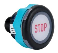
Captron Caneo Series10 Standard capacitive pushbutton sensor switch, IP69K, 22mm, static, polycarbonate bezel, semi-automatic LED control, Operator: white, 30mm, operator text "STOP", red. Requires 4-pin female M12 cable.
