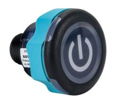
Captron Caneo Series10 Standard capacitive pushbutton sensor switch, IP69K, 22mm, static, polycarbonate bezel, semi-automatic LED control, Operator: black, 30mm, operator text "power symbol", green/red illuminated. Requires 4-pin female M12 cable.
