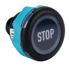
Captron Caneo Series10 Standard capacitive pushbutton sensor switch, IP69K, 22mm, static, polycarbonate bezel, semi-automatic LED control, Operator: black, 30mm, operator text "STOP", red/green illuminated. Requires 4-pin female M12 cable.
