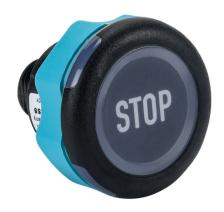
Captron Caneo Series10 Standard capacitive pushbutton sensor switch, IP69K, 22mm, dynamic, polycarbonate bezel, semi-automatic LED control, Operator: black, 30mm, operator text "STOP", red/green illuminated. Requires 4-pin female M12 cable.
