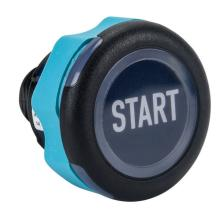
Captron Caneo Series10 Standard capacitive pushbutton sensor switch, IP69K, 22mm, static, polycarbonate bezel, semi-automatic LED control, Operator: black, 30mm, operator text "START", green/red illuminated. Requires 4-pin female M12 cable.
