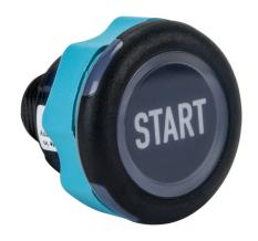
Captron Caneo Series10 Standard capacitive pushbutton sensor switch, IP69K, 22mm, dynamic, polycarbonate bezel, semiautomatic LED control, Operator: black, 30mm, operator text "START", green/red illuminated. Requires 4-pin female M12 cable.
