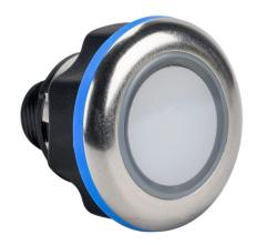
Captron Caneo Series10 Hygienic capacitive pushbutton sensor switch, IP69K, 22mm, static, stainless steel bezel, semi-automatic LED control, Operator: white, 32.4mm. Requires 4-pin female M12 cable.
