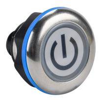
Captron Caneo Series10 Hygienic capacitive pushbutton sensor switch, IP69K, 22mm, static, stainless steel bezel, semi-automatic LED control, Operator: white, 32.4mm, operator text "power symbol", black. Requires 4-pin female M12 cable.
