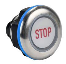
Captron Caneo Series10 Hygienic capacitive pushbutton sensor switch, IP69K, 22mm, dynamic, stainless steel bezel, semi-automatic LED control, Operator: white, 32.4mm, operator text "STOP", red. Requires 4-pin female M12 cable.
