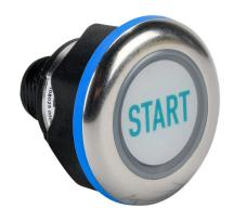
Captron Caneo Series10 Hygienic capacitive pushbutton sensor switch, IP69K, 22mm, static, stainless steel bezel, semi-automatic LED control, Operator: white, 32.4mm, operator text "START", green. Requires 4-pin female M12 cable.
