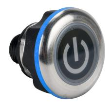
Captron Caneo Series10 Hygienic capacitive pushbutton sensor switch, IP69K, 22mm, static, stainless steel bezel, semi-automatic LED control, Operator: black, 32.4mm, operator text "power symbol", red/green illuminated. Requires 4-pin female M12 cable.
