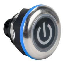
Captron Caneo Series10 Hygienic capacitive pushbutton sensor switch, IP69K, 22mm, static, stainless steel bezel, semi-automatic LED control, Operator: black, 32.4mm, operator text "power symbol", green/red illuminated. Requires 4-pin female M12 cable.
