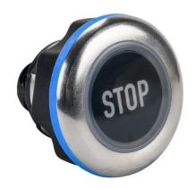
Captron Caneo Series10 Hygienic capacitive pushbutton sensor switch, IP69K, 22mm, static, stainless steel bezel, semi-automatic LED control, Operator: black, 32.4mm, operator text "STOP", red/green illuminated. Requires 4-pin female M12 cable.
