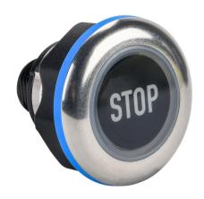
Captron Caneo Series10 Hygienic capacitive pushbutton sensor switch, IP69K, 22mm, dynamic, stainless steel bezel, semiautomatic LED control, Operator: black, 32.4mm, operator text "STOP", red/green illuminated. Requires 4-pin female M12 cable.
