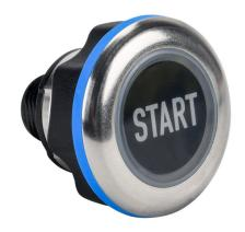
Captron Caneo Series10 Hygienic capacitive pushbutton sensor switch, IP69K, 22mm, static, stainless steel bezel, semi-automatic LED control, Operator: black, 32.4mm, operator text "START", green/red illuminated. Requires 4-pin female M12 cable.
