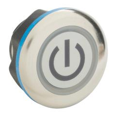
Captron Caneo Series10 Hygienic capacitive pushbutton sensor switch, IP69K, 22mm, static, stainless steel bezel, semi-automatic LED control, Operator: white, 32.4mm, operator text "power symbol", white.
