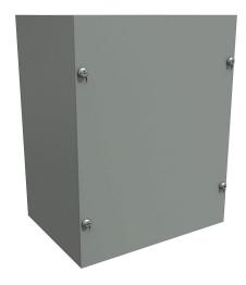
Hammond enclosure, NEMA 1, 10 x 8 x 6in (HxWxD), wall mount, carbon steel, ANSI 61 gray, powder coat finish, screw cover.
